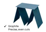
Cooling: dry Speed: 35 mm/min
