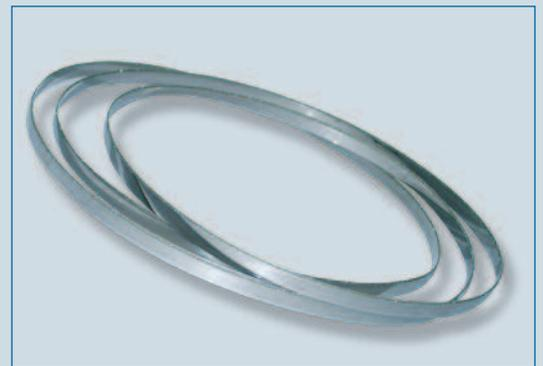
The saw band is 3200 mm long and 0.25 mm thick. It is an endless loop fitted with diamonds of grain-sizes D76, D126 or D181.
