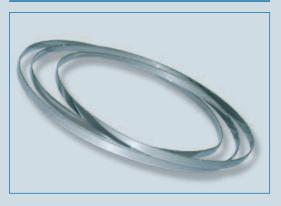
The saw band is 1870 mm long and 0.25 mm thick. It is an endless loop fitted with diamonds of grain-sizes D76, D126 or D181.
