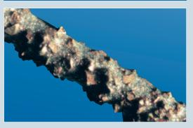
The cutting wire is 1870 mm long and 0.7 to 1.2 mm thick. It is formed as an endless, secure loop with diamonds of grain-sizes 76 - 181 µm. Precise movement of the wire is ensured because the flexible wire permits the use of small guiding rollers directly at the point to be worked.
